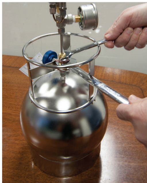
Proper use of wrenches to tighten fittings.
